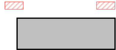
C.1: Laddering areas at adjacent corners of the longest side of the building.
