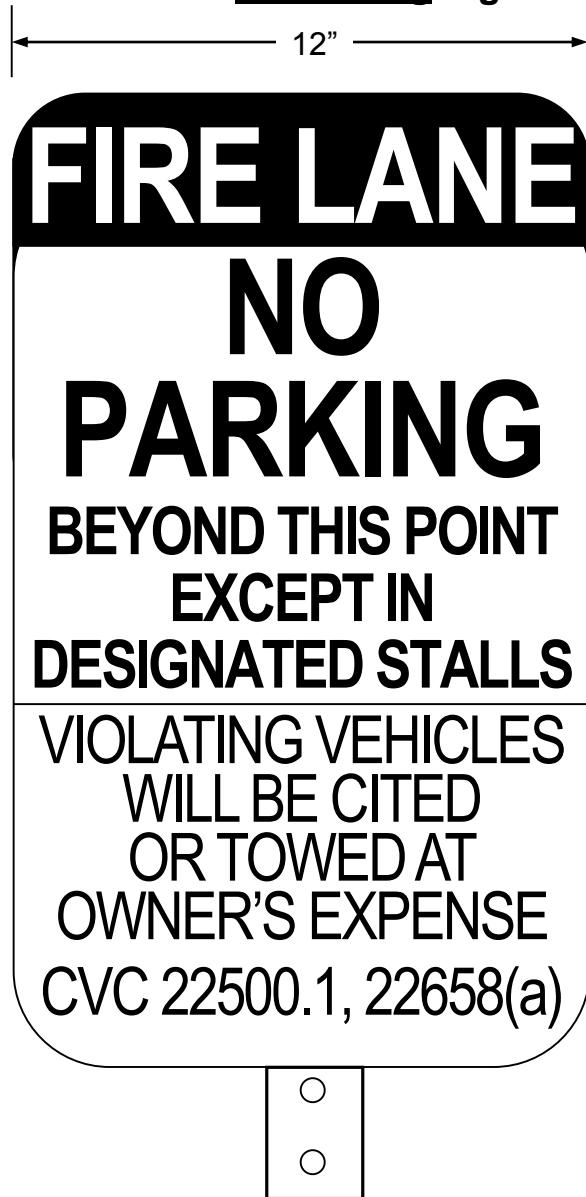
All sign and lettering dimensions shown are *minimums*. "Arial Narrow" font used in sample above, though other legible sans-serif fonts may be acceptable.
