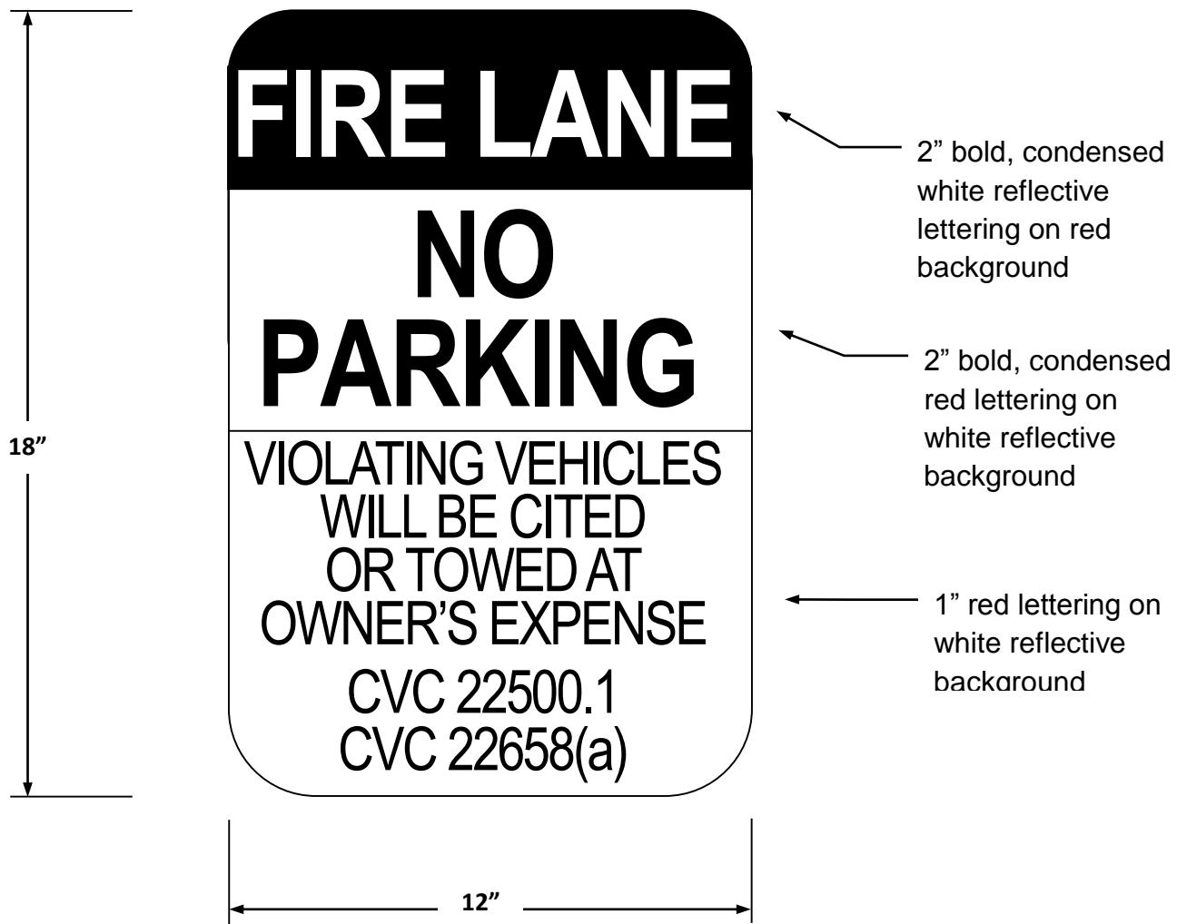
All sign and lettering dimensions shown are *minimums*. "Arial Narrow" font used in sample above, though other legible sans-serif fonts may be acceptable.
