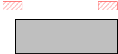
4.2.3.1. Laddering areas at adjacent corners of the longest side of the building.
