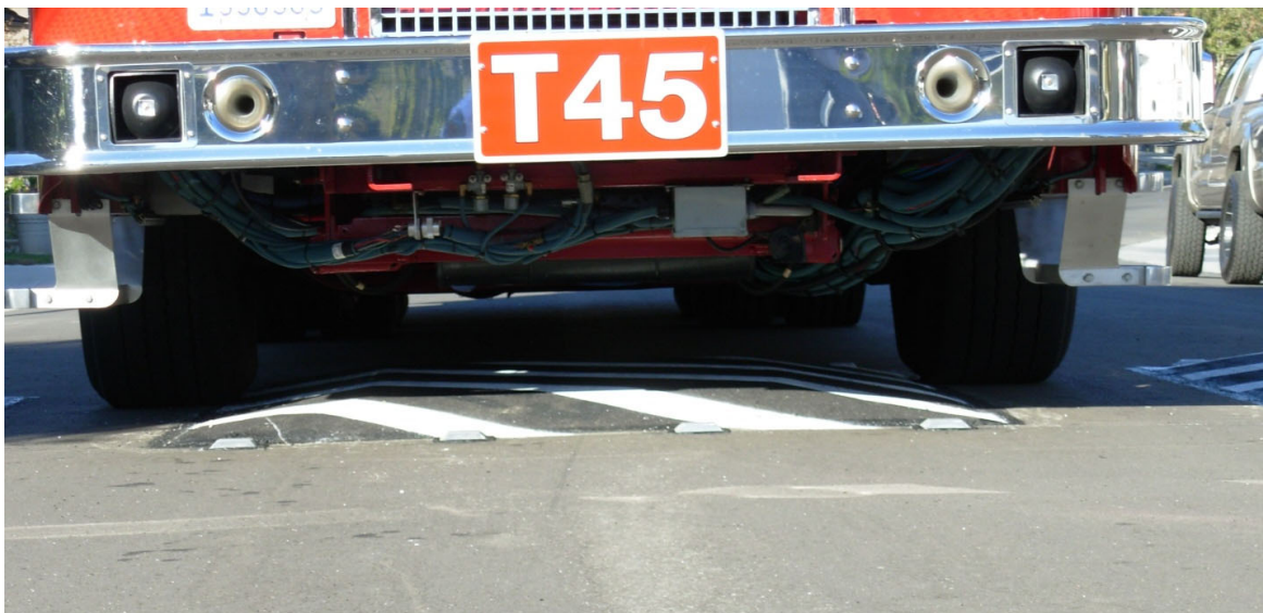
Figure 2: Fire truck straddling speed cushions. Locate the first speed cushion in the center of the street.
